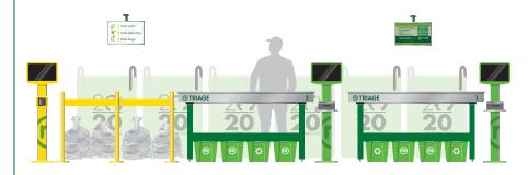
POS system concept showing count/sort tables, customer screens/terminals, printer for customer receipt, as well as the eventual addition of a drop & go recycling lane/terminal (shown here in yellow).
